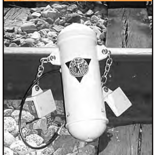
Picton Technology Ballast Integrity Sensor Model BIS-1 Dimensions: 6" diameter, 16" long
